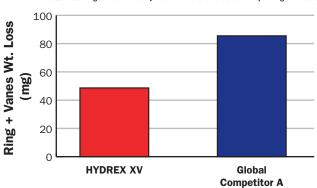
$^{\dagger}$ Test duration: 100 h/cartridge; Outlet pressure: 3200 psig; Inlet temperature: 104 °C (220 °F) Four ASTM D943 copper & iron coils added to reservoir for 200 h
